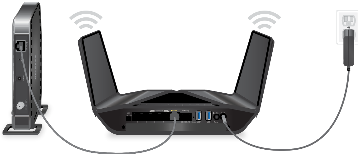
Figure 6. Cable your router
