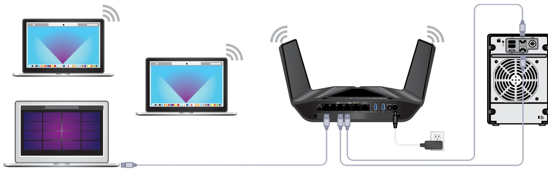
Figure 7. Ethernet port aggregation to a LAN device
