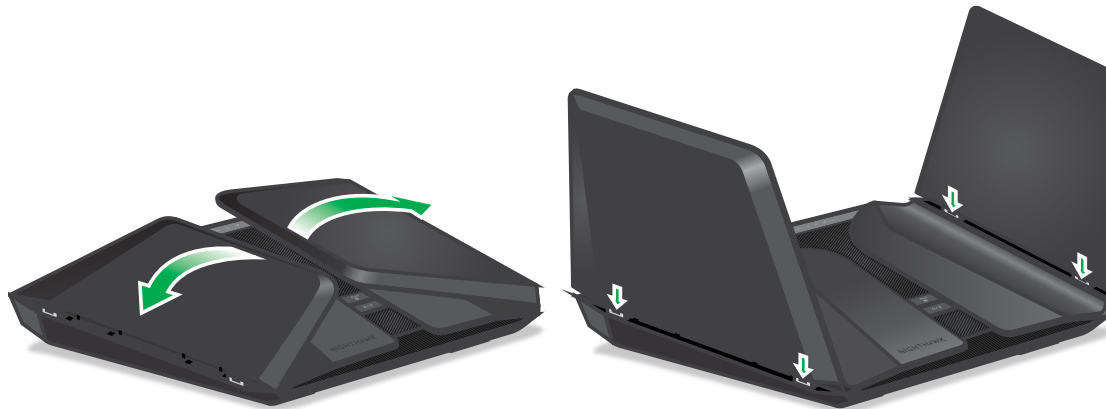
Figure 4. Position the antennas
